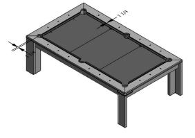
AFTER APPLYING COVER TO THE RAIL FRAME, LIFT IT IN PLACE ON THE TABLE. CENTER THE RAIL FRAME ON THE CHASIS AND LEGS. USE THE SCREWS YOU REMOVED IN THE FIRST STEP TO FASTEN THE RAIL FRAME TO THE
