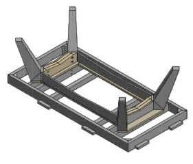
3 INSTALL THE CENTER STRETCHERS USING THE SCREWS AND ANGLE BRACKETS PROVIDED. THE STRETCHERS ARE FASTENED TO THE LEGS USING THE ANGLE BRACKETS.
