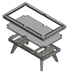
THE BASE IS NOW READY FOR THE INSTALLATION OF SLATE, BILLIARD CLOTH AND RAILS. REFER TO THE RAIL ASSEMBLY INSTRUCTIONS FOR INSTALLATION OF THE RAILS. HAVE A QUALIFIED TECHNICIAN INSTALL SLATE AND BILLARD CLOTH.
