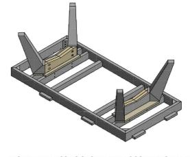
2 INSERT THE LEGS AS SHOWN AND LOOSELY INSTALL THE BOLTS AND WASHERS PROVIDED TO HOLD THE LEGS IN PLACE, BUT ALLOWING A LITTLE BIT OF MOVEMENT FOR INSTALLING THE CENTER STRETCHER.
